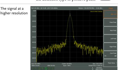
5. Press the **Detector** button and set the detection type to positive peak.
