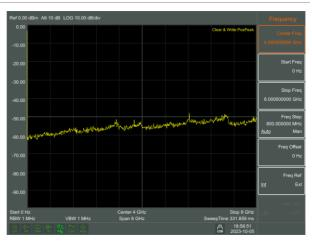
To clearly observe the signal, reduce the frequency span to 1 MHz and set the center frequency to 100MHz.
